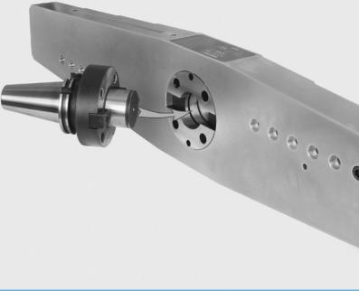
2.1 Fitted onto a milling cutter holder (flange mounting Type 569, spigot Ø 60 mm).
