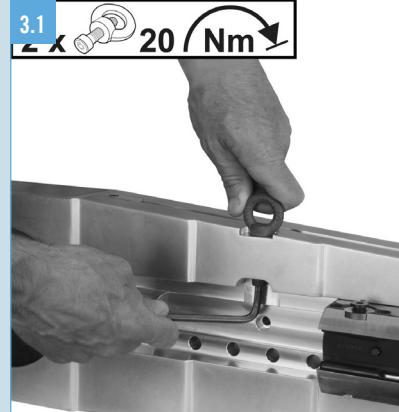
3.1 Fit the two lifting rings into Jumbo's lateral or back face, to be suitable for horizontal or vertical spindle fitting.
