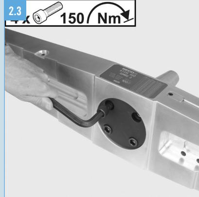
2.3 Locking the four Jumbo locking screws (tightening torque: 150 Nm).
