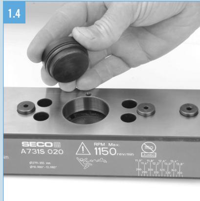
1.4 Place the sealing plug in central bore Ø 40 mm of each Bridge bar.
