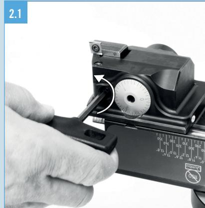
2.1. Before setting, unscrew of one revolution the barrel locking screw to unlock the micrometric adjusting system.
