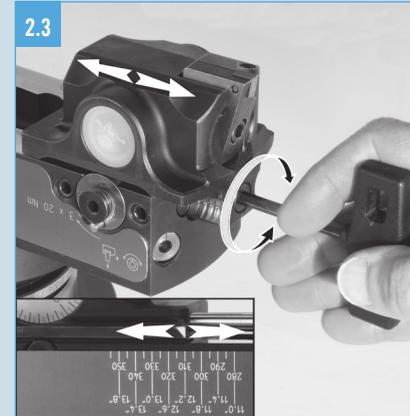
2.3. Preset fine boring block on required boring diameter.
