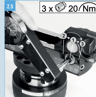
2.5 Tighten (tightening torque: 20 Nm) the stop disc screw and the two locking screws, on fine boring block and counterweight.
