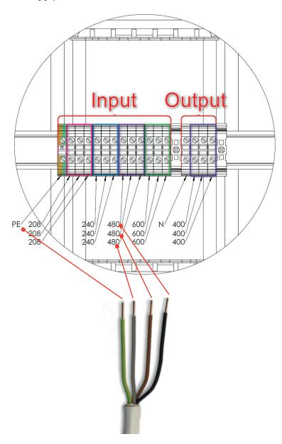
Don't forget to pass the cable through the hole in the door before connecting
